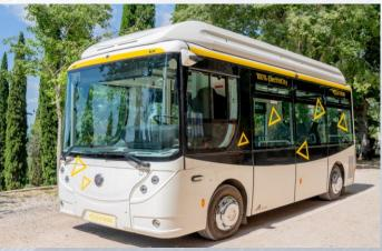
SIXTRON is a true Full Electric urban bus measuring 6 meters in length. Small on the outside and spacious inside, it's perfect for urban environments, with a low-floor platform and space for disabled passengers, accommodating up to 31 passengers. It's designed to operate with zero emissions, even in the narrowest alleyways of historic city centers.
